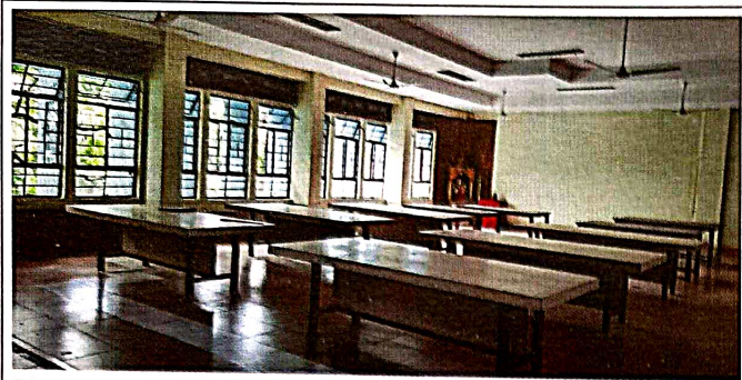
Figure 4: Classrooms with daylighting and WWR of up to 50%
