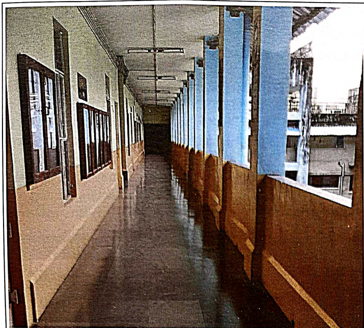
Figure 1: Classrooms banked by corridors prevent heat gain necessitating less use of energy for thermal comfort
